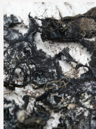
After being buried for six months, the nylon jersey fabric (left) remains relatively unchanged, whereas the wool jersey fabric (right) has significantly biodegraded.
